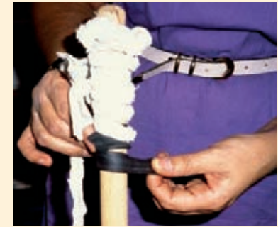
Work tools are made safer to hold, and grasp is facilitated, when handles are made larger and softer. Braided cloth and bicycle inner tubing are shown in this picture.
