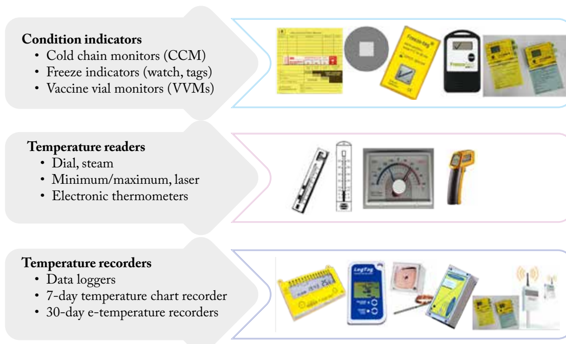
Figure 5.2 Categories of vaccine temperature monitoring devices
