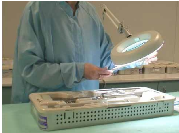
FIGURE 8: VISUAL INSPECTION OF A CLEAN SET 22
